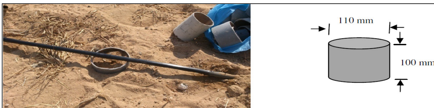
Fig. 4 : The best dimensions of PVC pipes cuts with pulse drip irrigation
